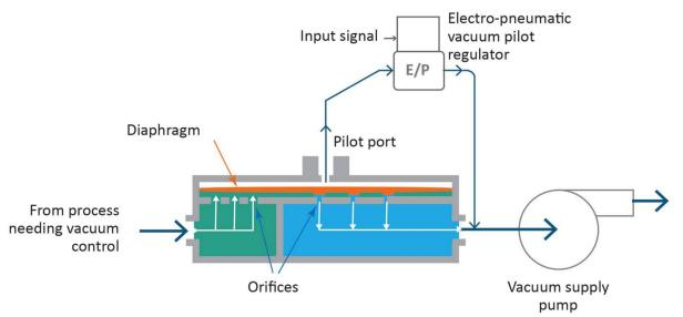
How it works schematic: A direct sealing diaphragm valve works in conjunction with an electro-pneumatic vacuum pilot regulator upstream of a vacuum pump. The diaphragm valve utilizes multiple orifices and vacuum pilot pressure on top of the diaphragm to adjust the diaphragm position to create precise vacuum control across a wide range of conditions.
